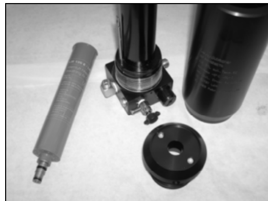
Filter cartridge & components of the filter housing
