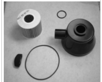
Ill.: 3 Inlet filter housing components and element
