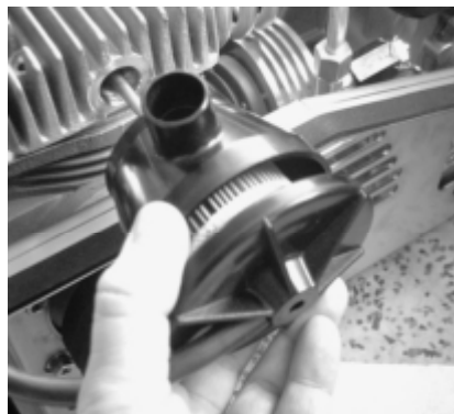
Ill.: 2 Unscrew the wing nut and remove the housing
