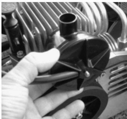
Ill.: 7 Fit the inlet filter housing carefully onto the 1st stage head and check the correct position (Air inlet up and vertical, crancase breather to the left)
