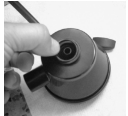
Ill.: 6 Fit the filter cartridge on the cover and place the housing over the element. Fit the O-Ring in the O Ring groove
