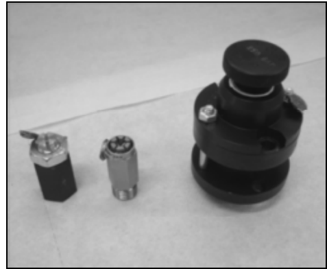
Safety valves (1st Stage / 2nd Stage / 3rd Stage)
