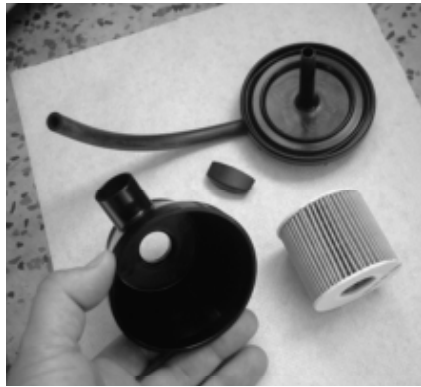
Ill.: 4 Clean the housing and inspect for damage ( cracks etc. ). Inspect the O Ring for damage
