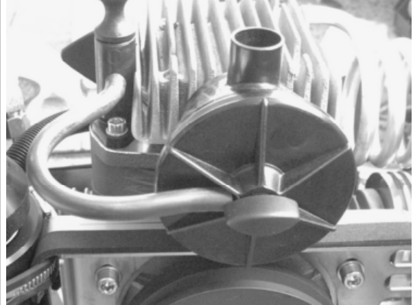
ill.: Crankcase breather hose and inlet filter housing
