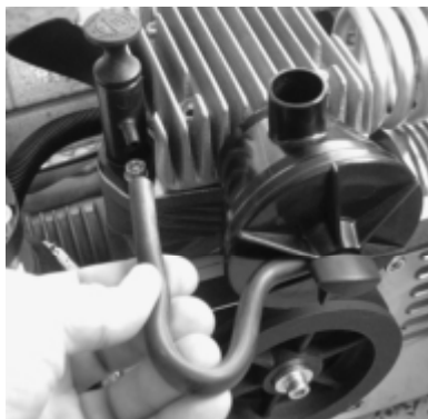
Ill.: 1 Remove the crankcase breather hose.
