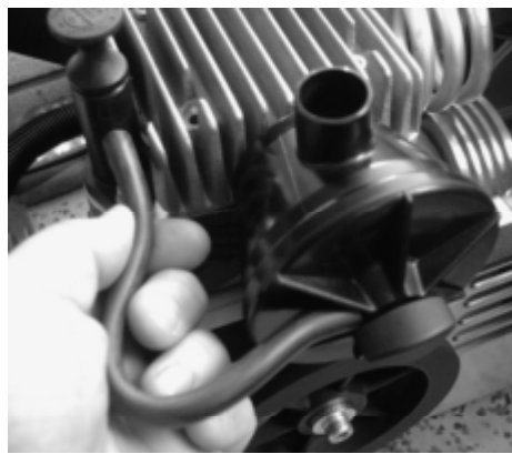
Ill.: 8 Fit and tighten the wing nut and refit the crankcase breather hose to the inlet filter housing and the oil filling neck
