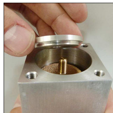
Fig. 5 - Place filter washer and washer
