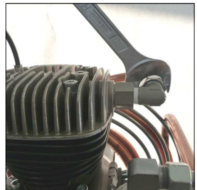
Fig. 6 - Connect pipe connections and tighten
