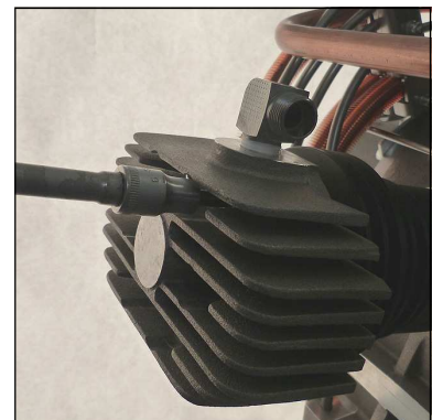
Fig. 2 - Loosen valve head screws
