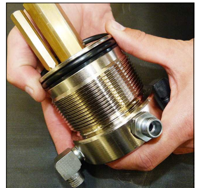
Fig. 4 - Change o-ring and back-up rings
