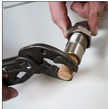
Fig. 3 - Change sinter filter
