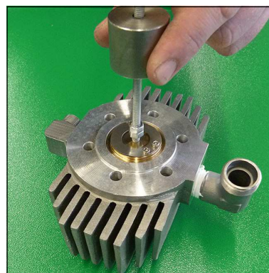
Fig. 4 - Remove inlet and outlet valve
