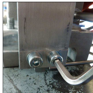
Fig. 1 - Loosen mounting screws
