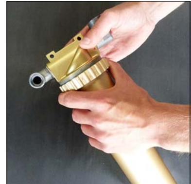
Fig. 1 - Open ring nut and remove separator top
