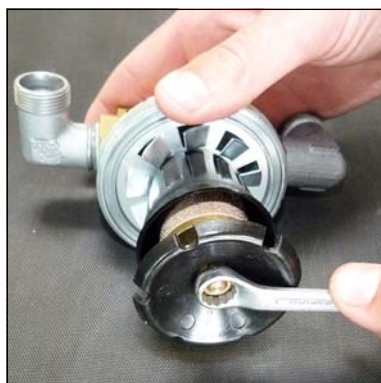
Fig. 2 - Loosen nut at the separator top
