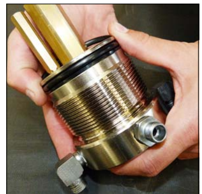
Fig. 4 - Change o-ring and back-up rings
