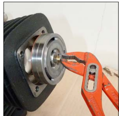
Fig. 2 - Pull out inlet and outlet valve
