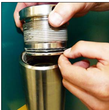
Fig. 2 - Change o-ring and back-up rings
