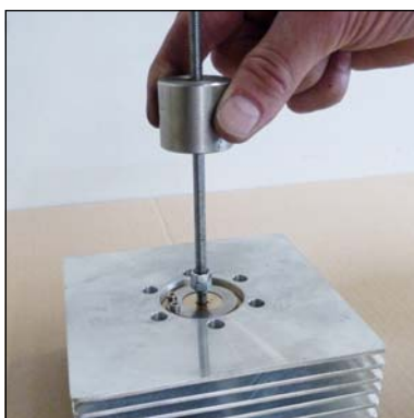
Fig. 3 - Remove inlet and outlet valve
