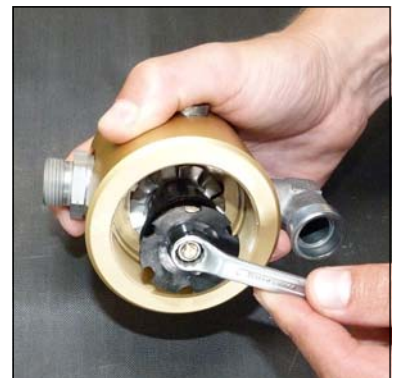
Fig. 2 - Loosen nut at the separator top
