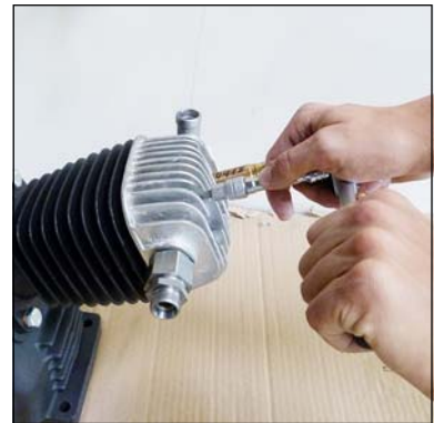
Fig. 1 - Loosen valve head screws
