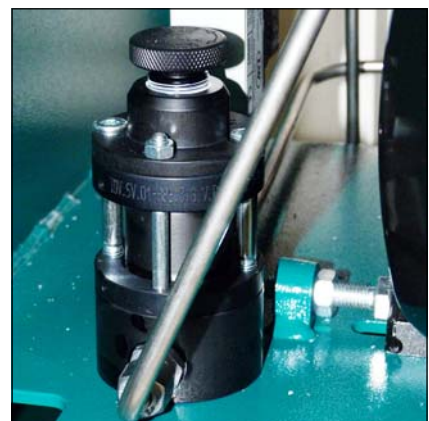
Safety valve 3rd stage
