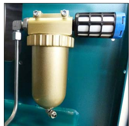
Oil / water separators final stage
