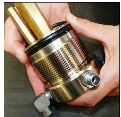
Fig. 4 - Change o-ring and back-up rings
