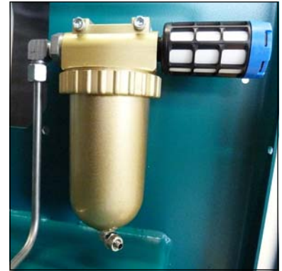
Oil / water separators final stage
