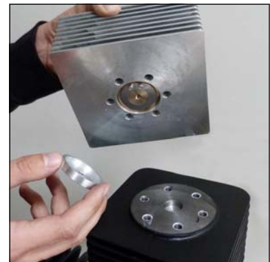
Fig. 2 - Remove lower valve gasket
