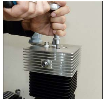
Fig. 1 - Loosen valve head screws
