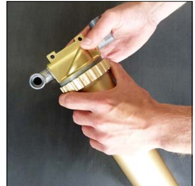
Fig. 1 - Open ring nut and remove separator top
