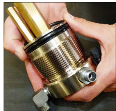
Fig. 4 - Change o-ring and back-up rings
