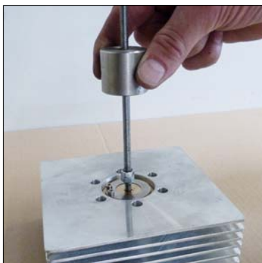
Fig. 3 - Remove inlet and outlet valve
