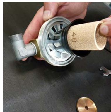
Fig. 3 - Change sinter filter
