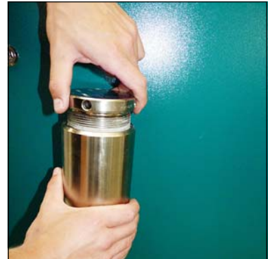
Fig. 1 - Open Filter cover
