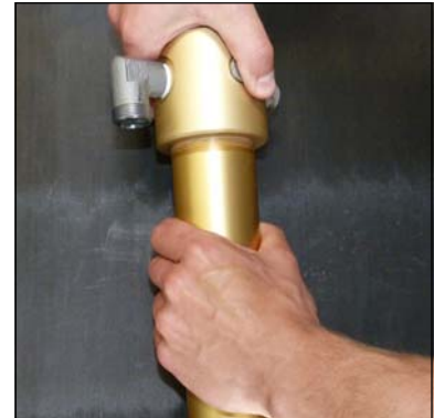
Fig. 1 - Unscrew and remove filter top
