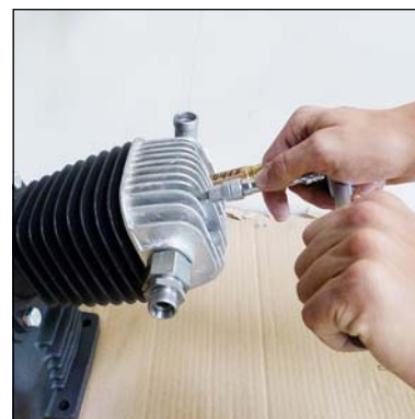
Fig. 1 - Loosen valve head screws
