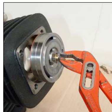
Fig. 2 - Pull out inlet and outlet valve
