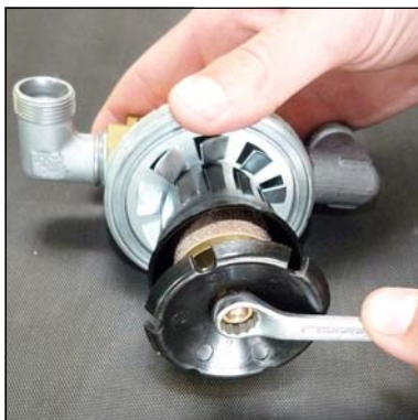
Fig. 2 - Loosen nut at the separator top
