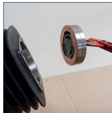
Fig. 3 - Place new inlet and outlet valve straightly into cylinder
