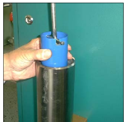
Fig. 3 - Pull the cartridge out of the housing.
