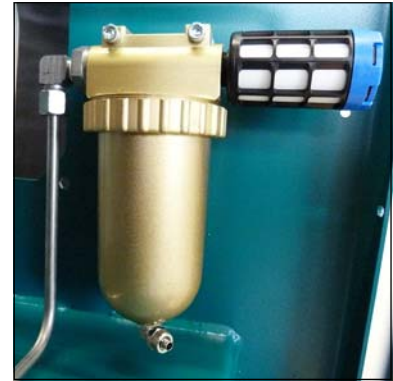
Oil / water separators final stage
